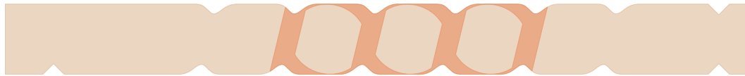
Figure 2.1: The \mu\text{F} actuator strip pattern with three SMA active elements presented in the M.S. thesis
